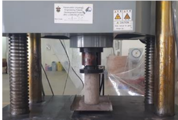
Figure 2. Compressive strength test method.
