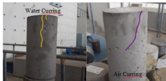
Figure 5. Crack pattern of 3 days geopolymer mortar.
