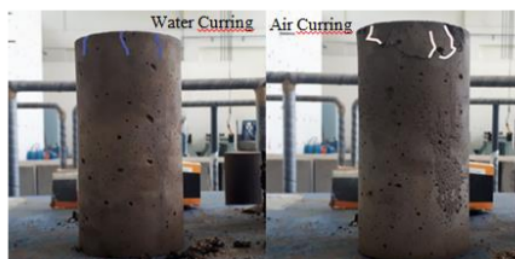
Figure 6. Crack pattern of 7 days geopolymer mortar
